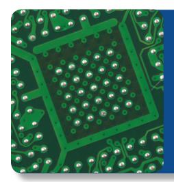
85NT is a pure polyimide laminate and prepreg system (Tg=250°C), reinforced with a non-woven aramid substrate. 85NT combines the high-reliability features of polyimide (improved PTH reliability and temperature stability) with the low in-plane (X,Y) expansion and outstanding dimensional stability of the aramid reinforcement.
